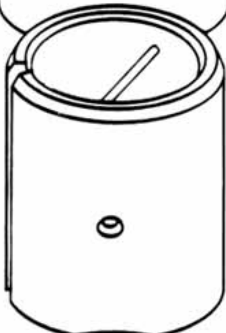
Internal Tension Bush (EG) with closed internal grease groove pattern and lubrication holes for radial lubrication application
