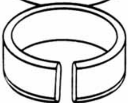
Internal Tension Bush (EG) with rounded edge
