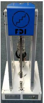
Tensile Frame: This unit is designed for testing test specimens or threaded parts in tension using either the RSL method or standard tensile loading parameters. It is capable of exerting tensile forces up to 10,000 pounds. This tensile frame is a single unit device meaning that the load control and scientific controller are all contained internally in the system.
