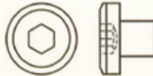
Hex Socket Low Head Cap Screw
